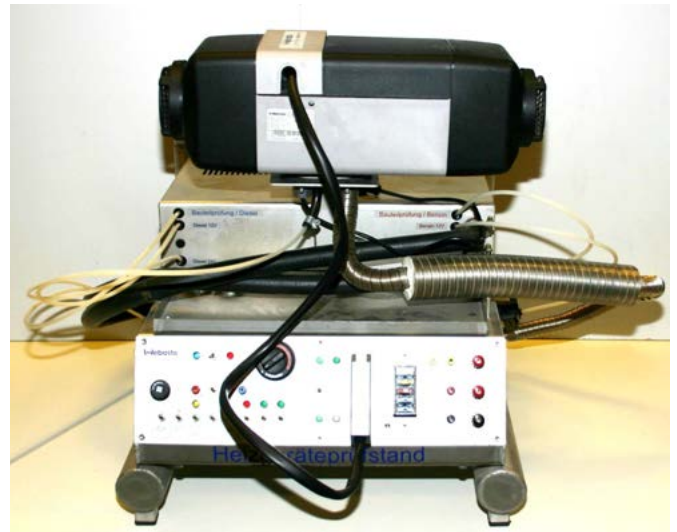
Example of heater test bench
